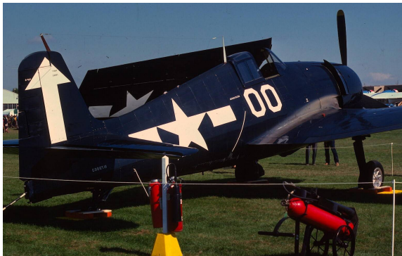
Hellcat Demonstrates Leroy Grumman's Unique Wing Folding Method.
